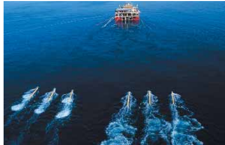
PGS Ramform seismic vessel utilizing Teledyne hydroacoustic streamer.
