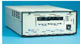
Air quality monitoring instrument for sulphur dioxide.
