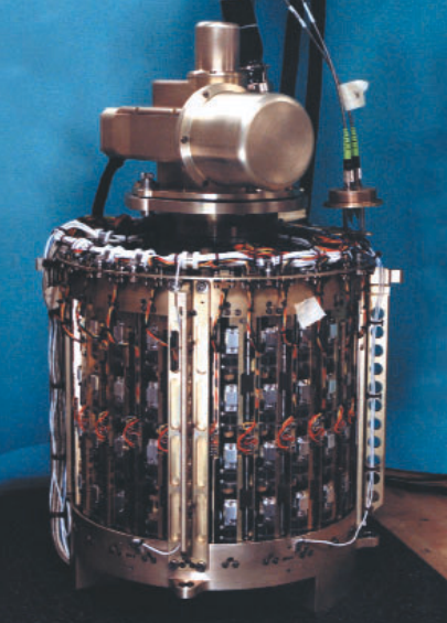
Teledyne Brown Engineering developed and space-qualified this Observable Protein Crystal Growth Apparatus for the University of California, Irvine
