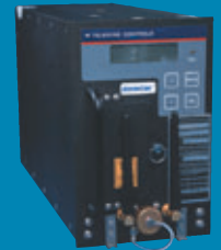
Wireless GroundLink™ automatically downloads flight information to an airline's operation center
