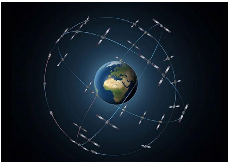
Representation of the Galileo global navigation satellites. 30 satellites in three MEO planes. The size of orbits relative to the Earth are approximately to scale but the satellites are depicted much larger than actual size. Credit: European Space Agency
