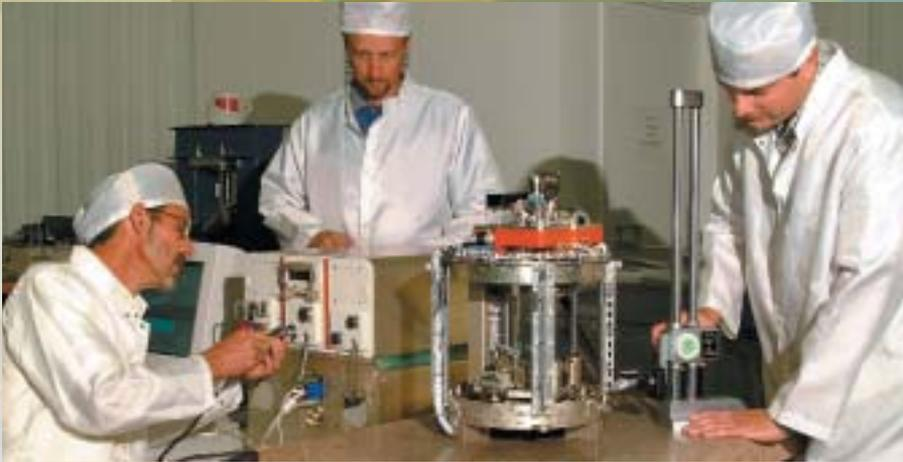
The Observable Protein Crystal Growth Apparatus is a device for the International Space Station that is used to delineate the relevant variables between Earth-grown crystals and Space-grown crystals.
